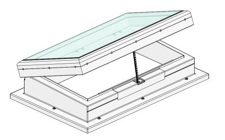
PLEASE NOTE: FLATLIGHT should be installed with a slope between 3° and 30° in order to avoid water pooling on the glass lid. All the upstands by TELFORM already include a standard 3° slope. Different pitch is available upon request.
